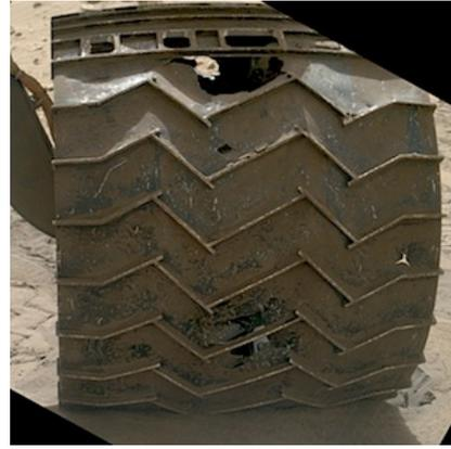
(a) Front HAZCAM on MER-B, sol 468, stuck in a 30cm sand dune (b) Damaged wheel on Curiosity, on sol 713. Several holes are visible in the wheel skin
